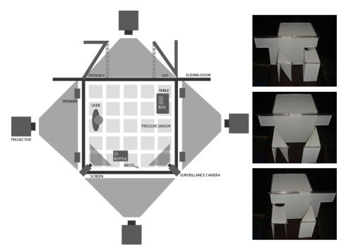
**Fig. 1.** Overview of "Eat me, drink me" stage. (a) left, the schematic overview of the physical setting (b) right, the scale model of the CAVE, from top to bottom: (1) the entrance is opened, (2) the entrance and exit are closed, (3) the exit is opened
