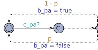
Fig. 5: Environmental modelling. In the figure  $p = 1 - \gamma_{Succ}(p_a)(p_a)$ .
