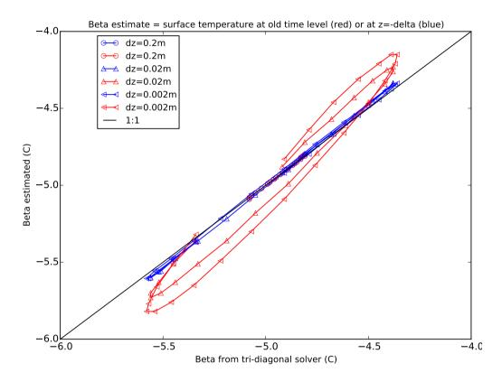
Figure 4. Empirical estimates of parameter  $\beta$  as a function of the value found from the tri-diagonal solver. The red curve represents the estimate according to  $T_1^n$  and the blue curve is the temperature at  $z = -\delta$ , also at the previous time level *n*. The symbols (connected by lines) indicate the successive time steps in the diurnal cycle. Results are plotted for vertical resolutions of 0.2, 0.02 and 0.002 *m*.
