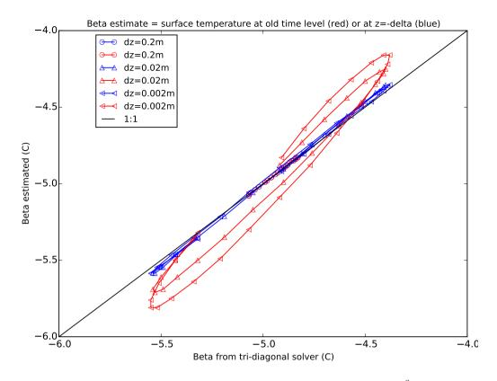
**Figure 7.** Dimensionless  $\beta$  as in Fig. 4, but for non-uniform snow density. The snow density is 150 kgm<sup>-3</sup> at the surface, increases linearly to 250 kgm<sup>-3</sup> at a depth of 0.5 m, and remains constant below 0.5 m.
