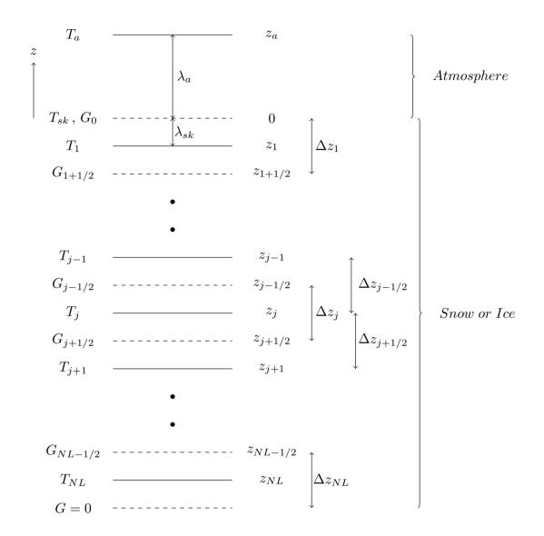
Figure 1. The numerical grid is defined by the position of the half levels, i.e. the thickness of the layers. The full levels are in the middle of the layers, i.e.  $z_j = (z_{j-1/2} + z_{j+1/2})/2$ . The surface is at z = 0. The bottom level is defined by the accumulated depth of all the layers. The temperature is defined on full levels and the heat fluxes are defined on half levels.
