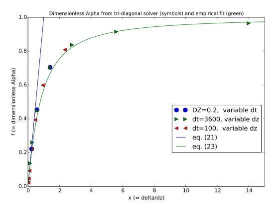
Figure 3. Dimensionless function  $f = \alpha (K \rho C / \Delta t)^{1/2}$  as a function of  $x = \delta / \Delta z$ . The circles and triangles are for different combinations of  $\Delta z$  and  $\Delta t$ . The blue line is the asymptotic limit for small  $\delta / \Delta z$ . The green curve is the empirical fit according to equation (22).
