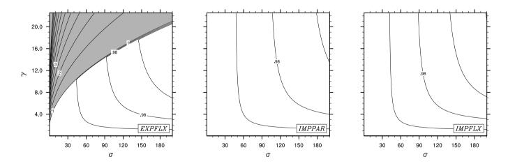
**Figure 8.** Spectral radius of the matrix  $\mathbf{M} = \mathbf{A}^{-1}\mathbf{B}$  (defined in B7,B8) associated to the explicit flux coupling (EXPFLX), parametrized implicit flux coupling (IMPPAR), and implicit flux coupling (IMPFLX) with respect to the dimensionless coefficients  $\gamma$  and  $\sigma$ . Gray shaded areas correspond to regions where the spectral radius is larger than 1.
