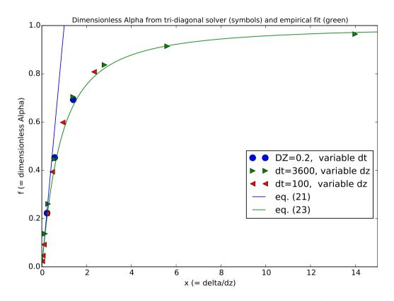
**Figure 6.** Dimensionless  $\alpha$  as in Fig. 3, but for non-uniform snow density. The snow density is 150 kgm<sup>-3</sup> at the surface, increases linearly to 250 kgm<sup>-3</sup> at a depth of 0.5 m, and remains constant below 0.5 m.
