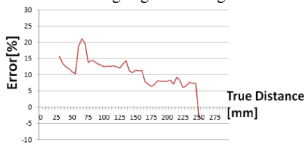
Fig. 11. Estimated error of distance between the HC2D barcode and the camera when the shooting angle is 30 degrees
