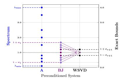
Figure 2: Spectrum Clustering for  $\hat{A}_i = A_i$ . The spectrum of some SPD matrix A and the transformations it goes after preconditioning by block Jacobi (BJ) and the WSVD preconditioner are displayed. The spectra are ordered from the left to the right starting from A, followed by BJ and ends up with WSVD.
