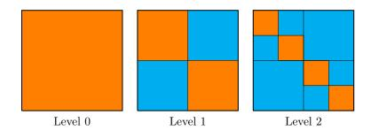
Figure 1: The HODLR Structure. The first 3 levels,  $\ell = 0, 1, 2$ , of the HODLR structure are illustrated: at each level the blue color blocks are the low rank blocks and the orange blocks are the HODLR principal submatrices of the level,  $A_k^{(\ell)}$ .
