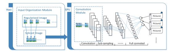
Fig. 1. Proposed GPU execution framework schematic.
