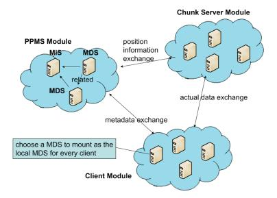
**Fig. 3.** Overview of PPFS. The system consists of three modules: PPMS module, chunk server module, and client module.
