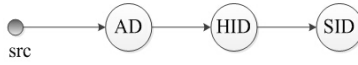
Fig. 4: An simple example of XIA address expressed in the DAG form ( src indicates a virtual source of DAG. AD is a 160-bits number identifying an AD. Similarly, HID and SID are 160-bits identifiers presenting a host or a service.)
