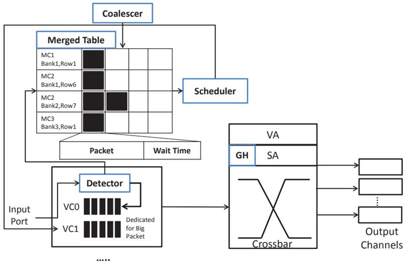
Fig. 1 The extended router microarchitecture for packet coalescing.
