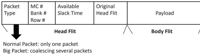
Fig. 2 Extended packet format for packet coalescing.
