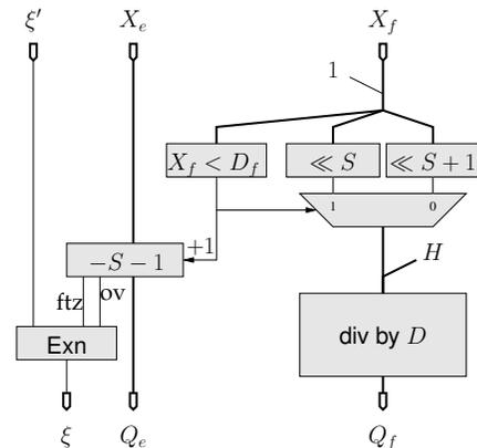
Fig. 10. Floating-point division by a small constant.
