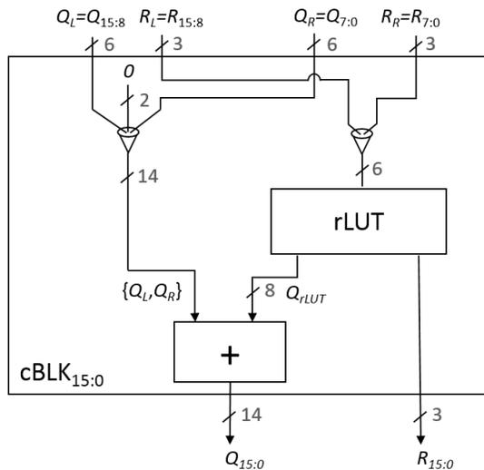
Fig. 6. Internals of  $cBLK_{15:0}$  of Fig. 5 (shaded)
