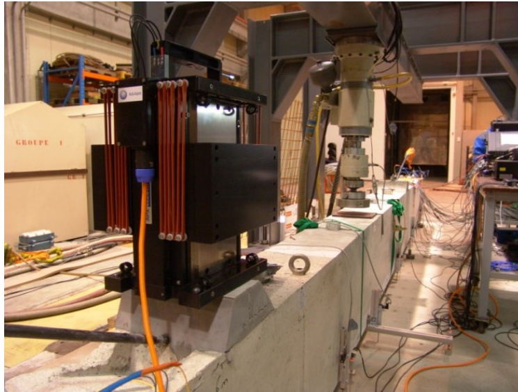
Figure 3: The specimen on the test bench with the shaker and the hydraulic jack.
