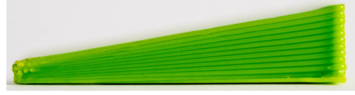
Figure 3: A slope generated by varying layer thicknesses across 12 layers. Each layer thickness varies from 0.07 mm to 0.38 mm uniformly from left to right. The nozzle width is 0.4 mm.
