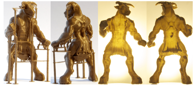
Figure 8: The minotaur. Left. Front and back view of the hollowed minotaur with support. Right. Front and back view of the backlit hollowed minotaur after support removal. One can see that the internal cavity has left material only in the feet, calves, hands, shoulders and head.
