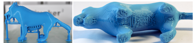
Figure 12: The wolf. Side view with our support structure and bottom view with support removed. The quality is equivalent to standard single-material support techniques.
