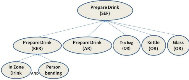
Fig. 4. Composite relations between concepts and event models. Multimodal Event “Prepare drink” is composed of conceptual events “prepare drink” from KER and AR detectors and conceptual objects “Tea bag”, “Kettle” and “Glass” from OR detectors. For instance, the hierarchically lower event “Prepare drink” from KER detector can be further decomposed into two sub-events, while other detector concepts are atomic.
