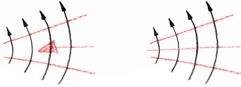
Fig. 7: Unit-norm vector fields with curl are not integrable; PGP gives a scalar field whose gradient is close to the given vector field. Left: integrating without cancelling the curl of the black field creates one singular triangle (highlighted in red). Red lines show integer iso-values of the scalar field, thus forming quads with the black lines (integer iso-values of the integrated orthogonal field). Right: integration with curl correction eliminates the singularity at the expense of introducing more distorted hexahedra.
