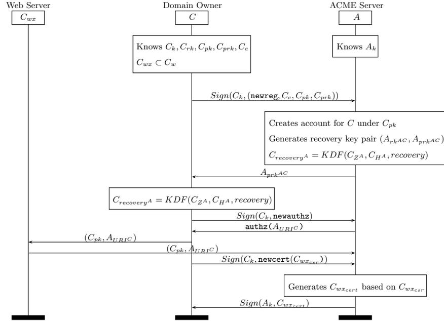
Fig. 4: ACME draft-1 protocol functionality for  $C$  account registration, recovery key generation, and validation with certificate issuance for  $C_{wx}$ . This chart demonstrates validation via an HTTP identifier. In draft-3 and above, the HTTP challenge  $(C_{pk}, A_{URIC})$  is replaced with  $Sign(C_k, (C_{pk}, A_{URIC}))$ .
