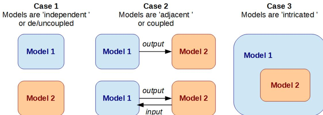
FIGURE 3. The three different types of hybrid models.
