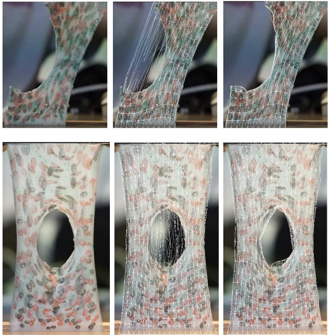
**Fig. 3** Detection and simulation of cuts in silicone bands demonstrating the ability of our approach to distinguish between large strains (186% and 166%) and cuts: left: without augmentation, right: augmented with an uncut/cut model.
