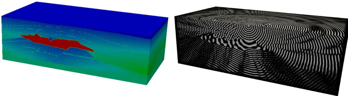
Figure 2: 3D SEG/EAGE salt dome velocity model: problem geometry with velocity distribution (left) and real part of numerical solution at 12 Hz (right). Figures from [26, Chapter 4].
