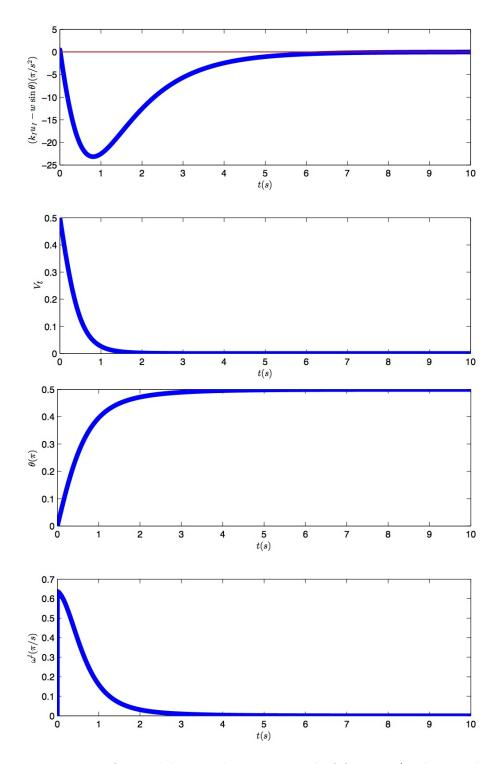
Figure 1: Perfect stabilization by PID control of  $\theta_{ref} = \pi/2$ , despite the action of the gravitational potential considered as a priori unknown. The parameters are w = 1, and we take  $b = 100, k_P = 1000, k_I = 1, k_D = 600$  to satisfy (4). The Lyapunov function is shown with  $\alpha = 1/k_P = 0.001$  and  $\beta = 1/(k_P * (b + k_I) * k_I) = 1/101000$ .
