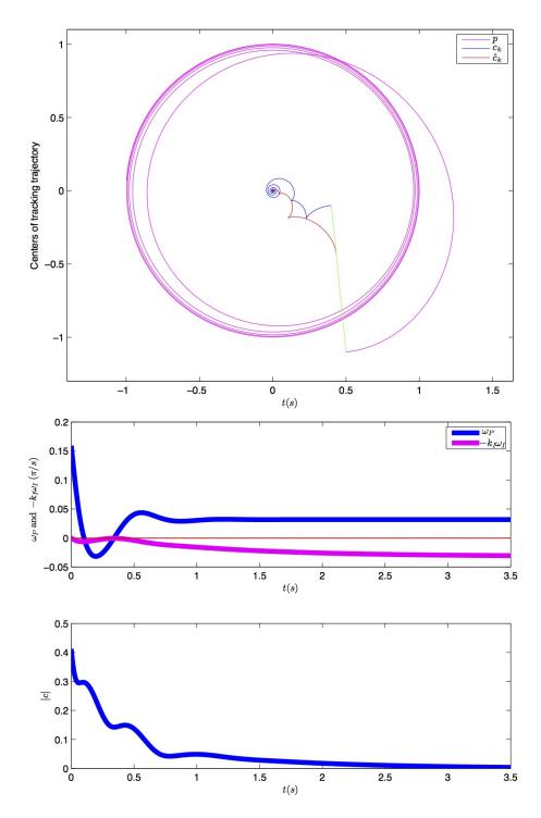
Figure 3: Same plots as on Fig.2, now including the adapted integral control (14) with  $k_I = 0.1$ . Since  $|v \sin \phi| = 0.1 = \tan \phi$ , one easily checks that the conditions (15) are satisfied. The vehicle now converges perfectly to the target trajectory, while the bias effect is countered by the integral control input.
