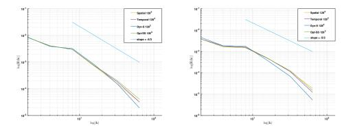
Figure 14: Wavelet energy spectrum at  $t \approx 9$  (left) and  $t \approx 14.7$  (right). Comparison between the three variance tensor models, the dynamic Smagorinsky model and the DNS solution. Taylor-Green vortex at Re = 5000 for a  $128^3$  mesh grid.
