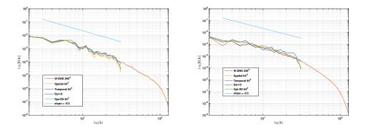
Figure 9: Total energy spectrum at  $t \approx 9$  (left) and  $t \approx 14.7$  (right). Comparison between the three variance tensor models, the dynamic Smagorinsky model and the DNS solution. Taylor-Green vortex at Re = 1600 for a  $64^3$  mesh grid.
