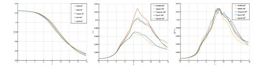
Figure 4: Evolution of the dimensionless energy  $\mathcal{E}(t)$  (left) and of the energy dissipation rate  $\epsilon_{\mathcal{E}} = -\frac{d}{dt}\mathcal{E}(t)$  (right) as a function of the dimensionless time. Comparison between the spatial covariance model, the dynamic Smagorinsky model and the wavelet DNS for the Taylor-Green vortex at Re = 1600 for a  $128^3$  mesh grid.
