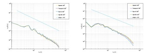
Figure 13: Total energy spectrum at  $t \approx 9$  (left) and  $t \approx 14.7$  (right). Comparison between the three variance tensor models, the dynamic Smagorinsky model and the DNS solution. Taylor-Green vortex at Re = 5000 for a  $128^3$  mesh grid.
