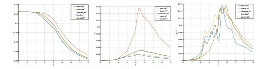
Figure 7: Evolution of the dimensionless energy  $\mathcal{E}(t)$  (left) and of the energy dissipation rate  $\epsilon_{\mathcal{E}} = -\frac{d}{dt}\mathcal{E}(t)$  (right) as a function of the dimensionless time. Comparison between the spatial covariance model, the dynamic Smagorinsky model and the DNS [15] for the Taylor-Green vortex at Re = 5000 for a  $64^3$  mesh grid.
