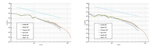
Figure 10: Total energy spectrum at  $t \approx 9$  (left) and  $t \approx 14.7$  (right). Comparison between the three variance tensor models, the dynamic Smagorinsky model and the DNS solution. Taylor-Green vortex at Re = 1600 for a  $128^3$  mesh grid.
