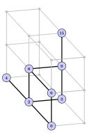
(a) Cray Gemini router from a 3D torus. One link on the *y*-axis is reserved to connect the compute nodes.
