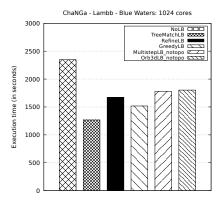
(a) Application walltime using different loadbalancers for the lambb use-case on for 512 cores (16 XE6 nodes) when varying the imbalance.
