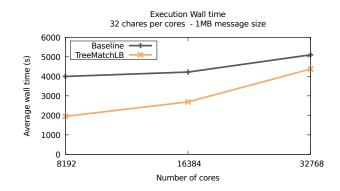
Figure 6: Average execution time of CommBench according to the number of cores with 32 chares per core and 1 MB per message. Carried out on XE6 nodes of the Blue Waters platform.
