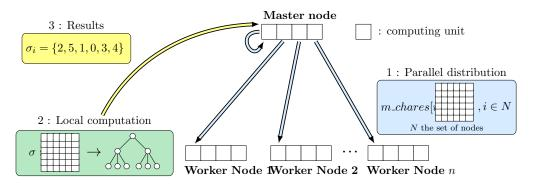
Figure 2: Master-Worker scheme of the Distributed Load Balancer
