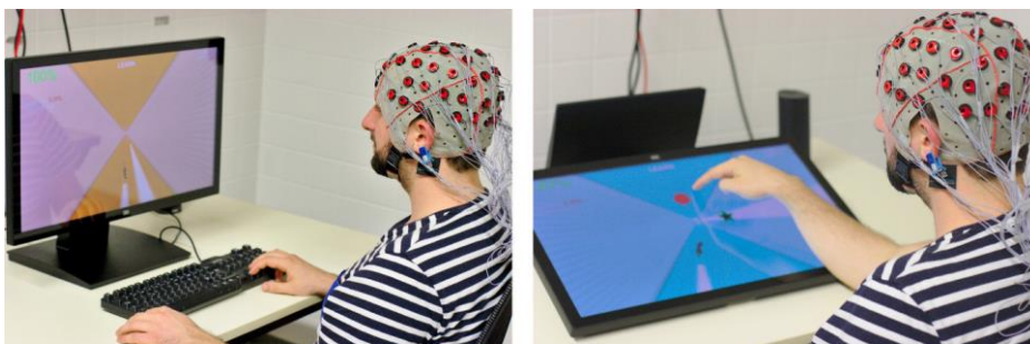
Figure 3. A keyboard and a touchscreen are compared using EEG measures during realistic interaction tasks.
