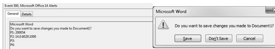
Figure 4. Microsoft Office Alert event generated by a prompt to save a modified file.
