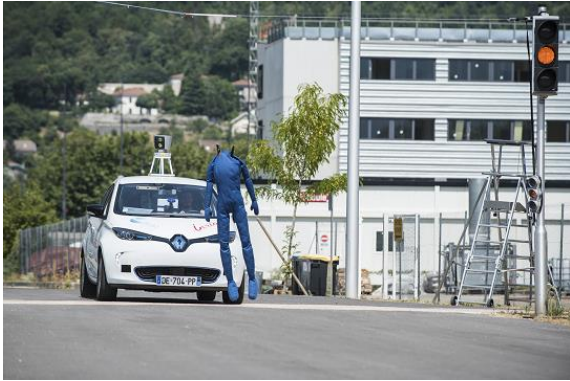
Figure 17: Risk collision experiments with our dummy crossing a street. © Inria / Photo H. Raguet.
