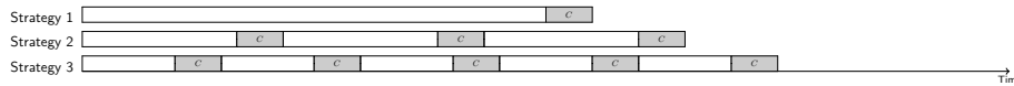
(a) Large MTBF: there are no or very few faults. Checkpointing is too expensive. The first strategy wins.
