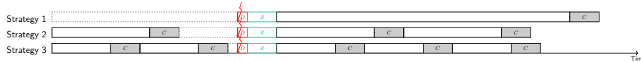
(b) Medium MTBF: there are more faults. It is good to checkpoint, but not too frequently, because of the corresponding overhead. The second strategy wins.
