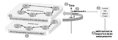
Fig. 2. Verification methodology mixing simulation and formal proof techniques.
