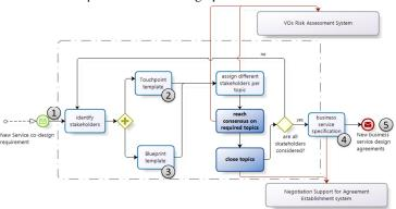
Fig. 3. Services co-design negotiation support system interactions.
