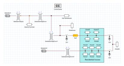
Figure 4: Smart grid CT model
