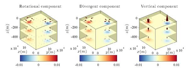
Figure 1: Value of the interior buoyancy created by a warm spot and a cold spot at the surface. The two components of the velocity are also shown. The upwelling and shrinking of the cyclone (cold spot) and the downwelling and spreading of the anticyclone (warm spot) are clearly visible.
