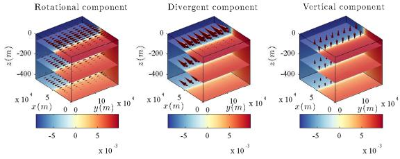
Figure 2: Value of the interior buoyancy created by a front at the surface. The two components of the velocity are also shown. The divergence effects will strengthen the front on the cold side (frontogenesis) and smooth the front on the warm side (frontolysis). The vertical velocity is here much weaker than in the case of isolated spots.
