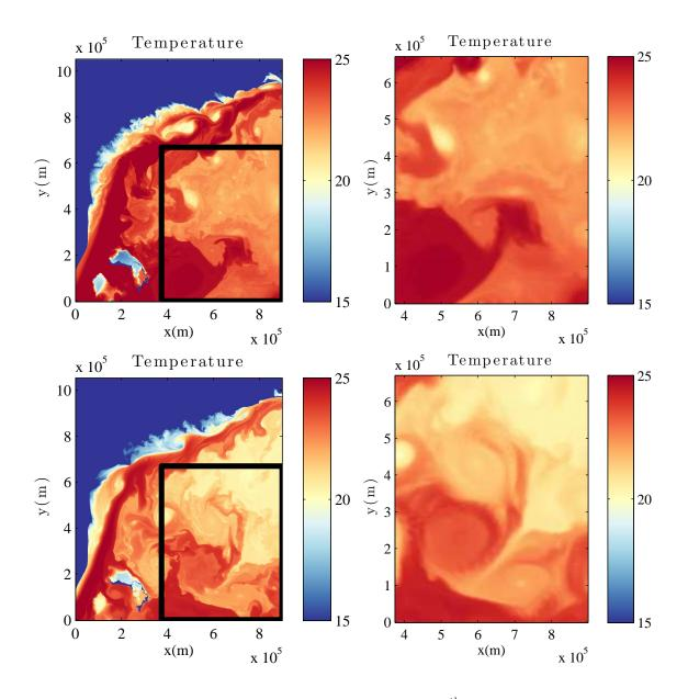
Figure 3: Temperature (in Celsius degree) for the first (top) and  $58^{th}$  day (bottom) at high temporal and spatial resolution ( $\Delta t = 12h$  and  $\Delta x = 750m$ ) (left) and after filtering ( $\Delta t = 1$  day and  $\Delta x = 3km$ ) (right). The black line on the top pictures highlight the region selected for the diagnostic.
