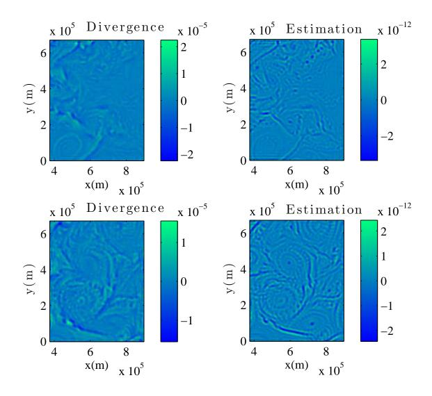
Figure 4: Divergence  $(s^{-1})$  and Laplacian of the vorticity  $(m^{-2}.s^{-1})$  for the first and the  $58^{th}$  day at a 30-km resolution. According to our modified geostrophic balance under strong uncertainty, the latter is an estimation of the mesoscale divergence up to a multiplicative constant.
