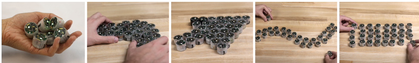
Figure 1. Zooids can be held as tokens, manipulated collectively or individually, behave as physical pixels, act as handles and controllers, and can move dynamically under machine control. They are building blocks for a new class of user interface we call swarm user interfaces .
