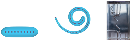
Figure 11: Data used for validation: capsule (left) and spiral (middle) surfaces and (right) the silicone vascular model. Both synthetic shapes presented respectively dimensions (width×height×depth) in mm: 11.9 \times 2.5 \times 2.5 and 8.1 \times 6.12 \times 1.05 . A primitive was placed at each red dot composing the skeleton (white).
