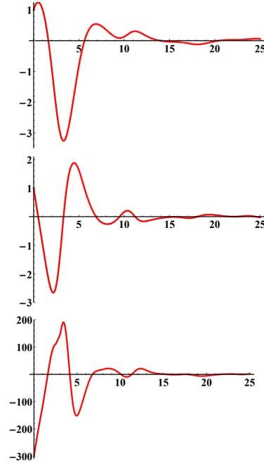
Fig. 2. Simulation of Nonlinear Pendulum Tracking System (44) with all Components of Initial Functions for  $x$  and the  $z_i$ 's set to 1 on  $[-1, 0]$  with Perturbation  $\delta(t) = 0$ . Top to Bottom:  $x_1(t)$ ,  $x_2(t)$ , and  $v(t-1)$  from (45).
