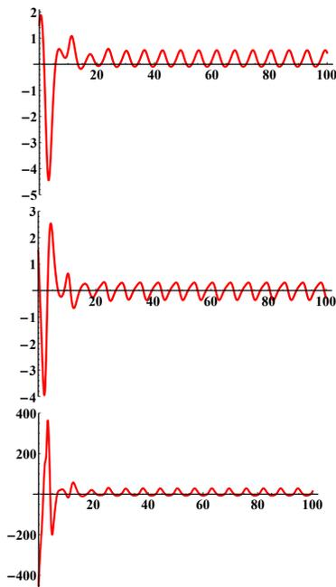
Fig. 4. Simulation of Nonlinear Pendulum Tracking System (44) with all Components of Initial Functions for  $x$  and the  $z_i$ 's set to 1.5 with  $\delta(t) = 0.05 \sin(t)$ . Top to Bottom:  $x_1(t)$ ,  $x_2(t)$ , and  $v(t-1)$  from (45).
