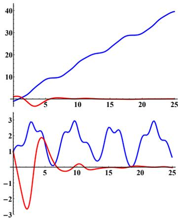
Fig. 3. Simulation of (44) from Fig. 2 (red) Showing Convergence, with Corresponding Simulations of Uncontrolled System Obtained by Setting  $u = \delta = 0$  in (44) (blue) Showing Divergence. Top to Bottom:  $x_1(t)$  and  $x_2(t)$ .
