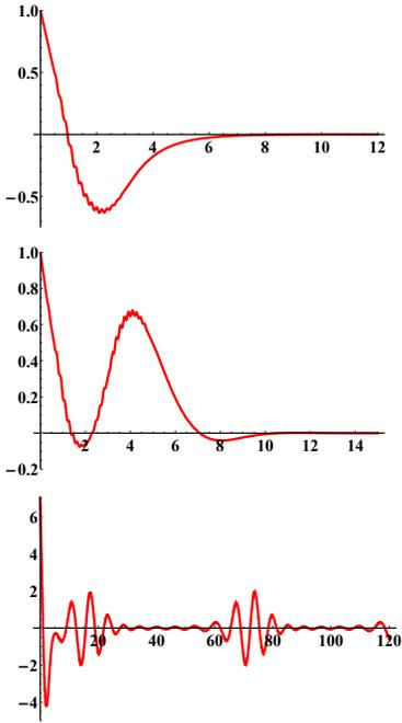
Fig. 1. Simulating  $x(t)$  for (35) with  $h = 1$  using Control (7) with  $m = 23$ ,  $k = 2$ ,  $\lambda_a = 0.0225$ , and  $x(r) = z_i(r) = \bar{x}$  for all  $i$  and  $r \in [-1, 0]$ , and Different Perturbations  $\delta$ . Top:  $\delta(t) = 0$  with  $\bar{x} = 1$ . Middle:  $\delta(t) = e^{-t} \sin(t)$  with  $\bar{x} = 1$ . Bottom:  $\delta(t) = 0.1 \sin(t)$  with  $\bar{x} = 7$ .
