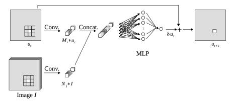
Figure 3: One enhancement iteration represented as common neural network layers.
