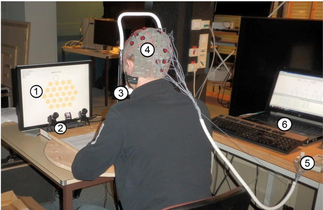
**FIGURE 2 | Experimental setup.** 1, Visual display; 2, Gaze tracker; 3, Chin rest; 4, EEG headset; 5, EEG signal amplifier; 6, Laptop with Openvibe software for EEG signal processing.
