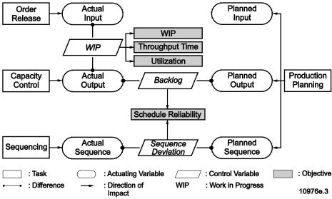
Fig. 1. A manufacturing control model [13]
