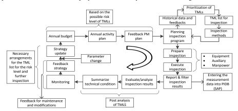
Fig. 1. Inspection planning work process
