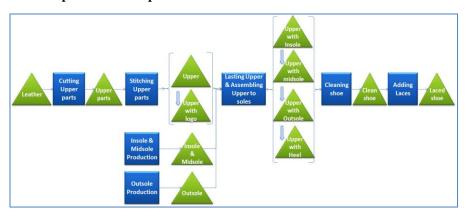
Fig. 4. : Simplified shoe fabrication process
