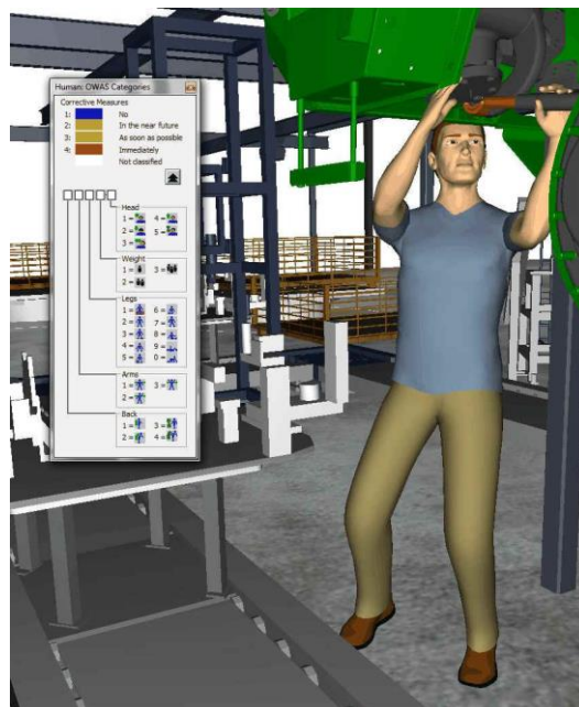
Fig. 3. Evaluation of overhead work using the OWAS method [3, p. 20; Software: 6]
