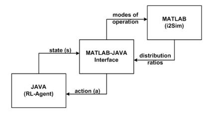
Figure 4. MATLAB-Java dependency diagram.
