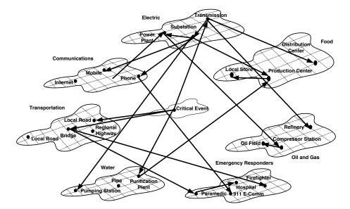
Figure 1. Interconnected critical infrastructures.
