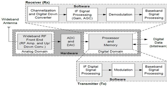
Fig. 2. SDR architecture for Relay Node [9].
