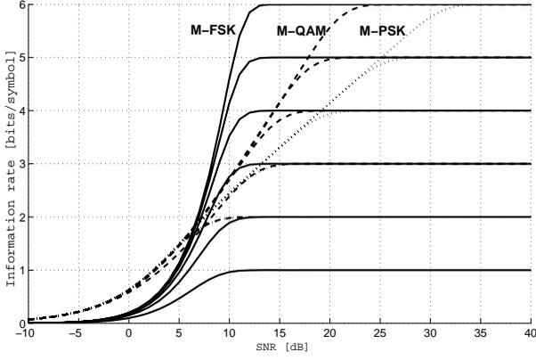
Fig. 4. Capacities and cutoff rates of MQAM, MPSK, and MFSK in AWGN channel as a function of predetection SNR. Each curve represents a different constellation size. The curves  $1 \leq \log_2 M \leq 6$  for M-FSK, and  $2 \leq \log_2 M \leq 6$  for M-QAM and M-PSK are shown, where  $M$  is the constellation size.
