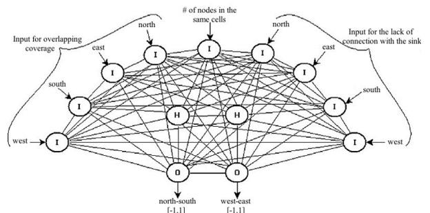
Fig. 3. Neural network architecture of one node
