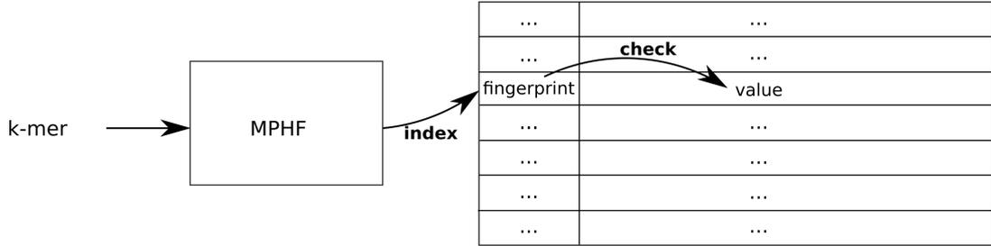
**Figure 1.** Quasi dictionary structure composed of a MPHF and a table of fingerprints. The fingerprints are obtained by hashing the corresponding  $k$ -mers. Thanks to the MPHF a unique index is associated to each  $k$ -mer where the fingerprint is stored. The fingerprint is associated to the value we want to link to the  $k$ -mer. When a  $k$ -mer is queried the fingerprint obtained is checked against the fingerprint stored to limit false positives.
