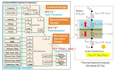
ITVs influence the module designs. Each module is designed to satisfy a target ITV using the internal design variables.
