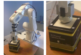
Fig. 5. The anthropomorphic robotic system equipped with a motorized 3D US probe and the ultrasound phantom.
