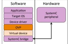
Fig. 2. Co-simulation architectures. Pink boxes indicate unchanged code between QEMU and OVP.
