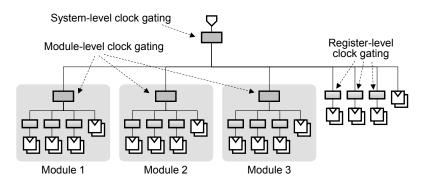
Fig. 4: Clock gating in multiple levels.
