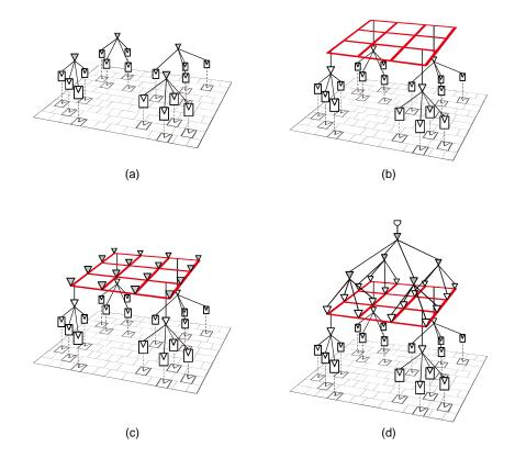
Fig. 3: Mesh clock network synthesis: (a) postmesh buffer insertion, (b) mesh grid construction, (c) mesh driver insertion, and (d) premesh tree synthesis.
