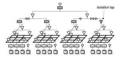
Fig. 6: Multiple mesh implementation of multi-level clock gating.
