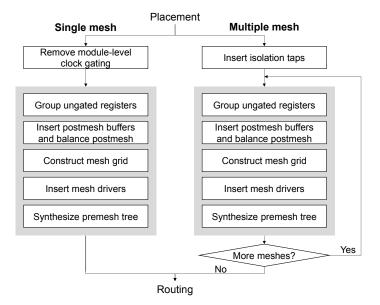
Fig. 7: Design flow of mesh network synthesis.
