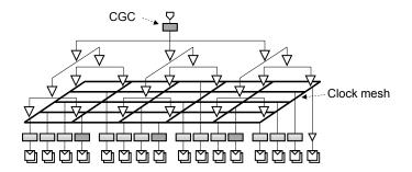
Fig. 5: Single mesh implementation of multi-level clock gating.
