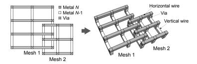
Fig. 14: Three-dimensional illustration of overlapped clock meshes.
