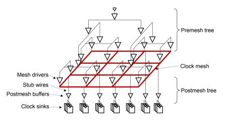
Fig. 2: Mesh clock network.
