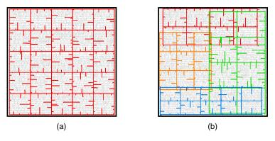
Fig. 8: Layouts of (a) single- and (b) multiple-mesh implementations for circuit ac97.
