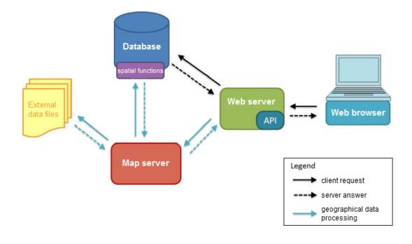
Figure 9: Software setup for online interactive maps to be dynamically linked to a database
