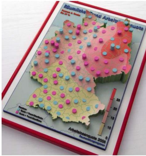
Fig. 5. Bivariate trend surface (order 5) and color-coded cylinders representing the values of the residuals. Cyan: residuals are negative (actual values less than the surface values); magenta: residual values are higher than the trend surface.
