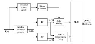
Figure 2. New block diagram for SVAC audio encoder
