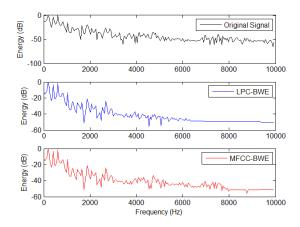
Figure 3. Reconstructed high-frequency spectrum in two encoders
