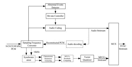
Figure 1. SVAC audio encoder block diagram
