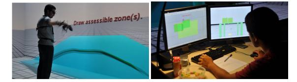
FIGURE 12 – Interfaces of the end-user and the design engineer : (left) end-user drawing their reachable zone on the table, (right) design engineer having two viewpoints on their workstation.
